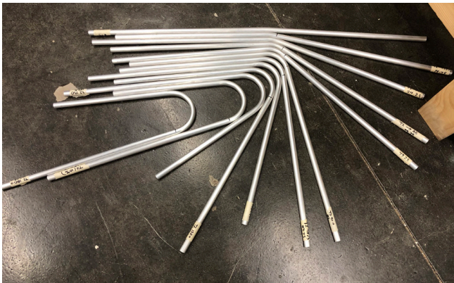
Figure 4. Twelve test bends ranging from 5-180 input degrees were executed in order to calibrate for material behaviour in terms of the desired bend angle, resultant bend angle, and springback. Image credit Authors.
