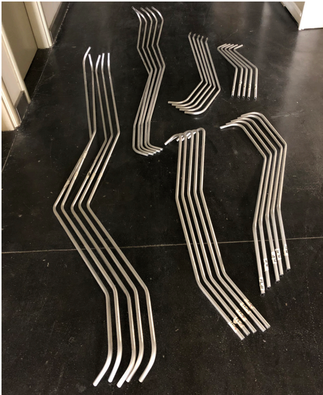
Figure 8. The multiplanar bent tube components that form InterLattice. Image credit Authors.
