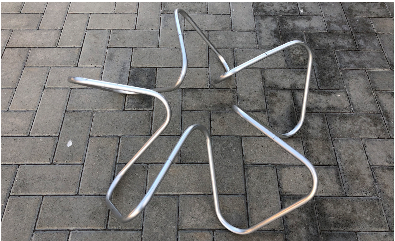
Figure 7. The completed initial prototype served to test accuracy of the developed workflow in three-dimensions while doubling as the structural table base. Image credit Authors.
