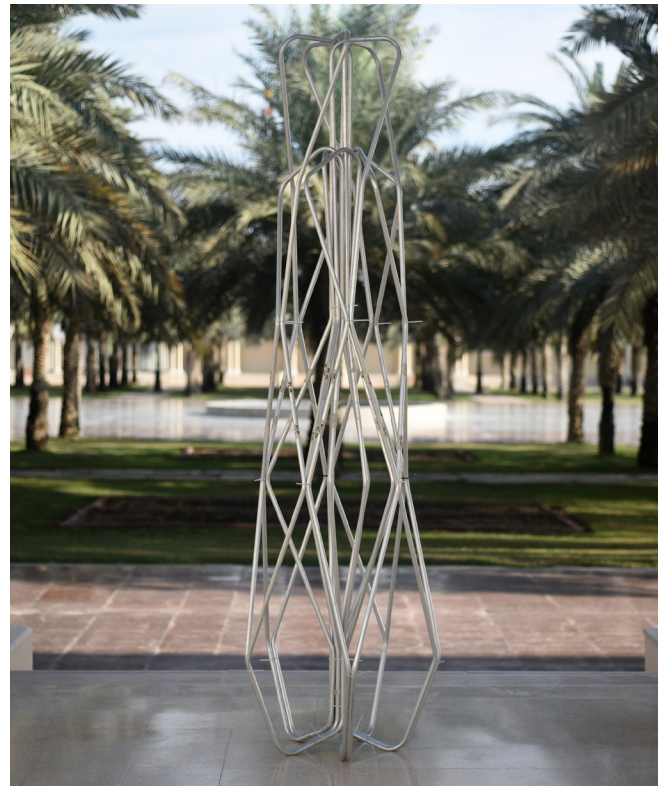
Figure 9. Test fitting of InterLattice loops shown with raw aluminum finish and temporary connections. Image credit Authors.
